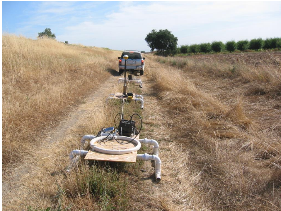
Figure 12 - Geonics Ltd. EM34 EM induction instrument being towed by a vehicle collecting continuous data (Llopis and Simms, 2007)
